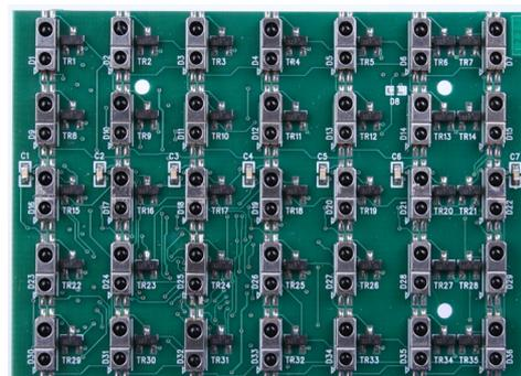
Figure 3: The front side of the sensor PCB showing the 7x5 array of IR optosensors. The transistors that enable each detector are visible to the right of each optosensor. Three such PCBs are used in our ThinSight prototype.
