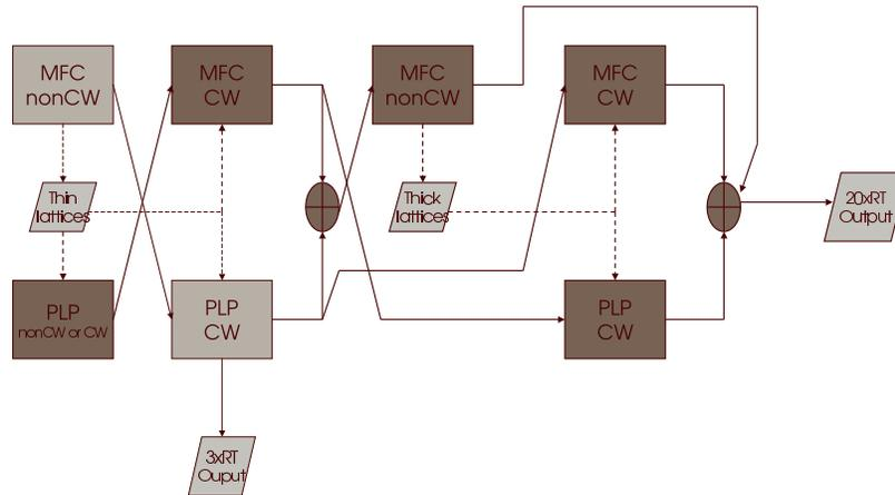
**Fig. 1.** SRI CTS recognition system. Rectangles represent decoding steps. Parallelograms represent decoding output (lattices or 1-best hypotheses). Solid arrows denote passing of hypotheses for adaptation or output. Dashed lines denote generation or use of word lattices for decoding. Crossed ovals denote confusion network system combination steps.
