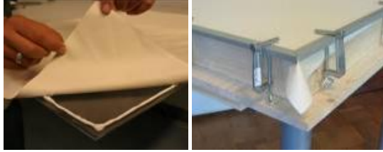
Figure 3: Building steps. Left: pouring an even distribution of the black liquid onto the acrylic and placing the latex sheet on top. Right: sealing panel with aluminum frame and silicon sealant.
