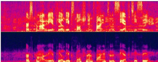
Figure 6. Spectrograms of the original data. Top: close-talk signal. Bottom: bone signal.
