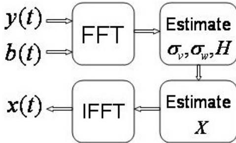
Figure 2. The direct filtering algorithm
