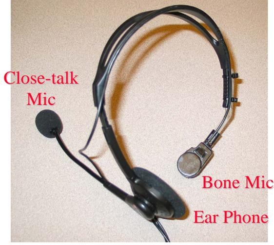
Figure 1. A WITTY microphone prototype
