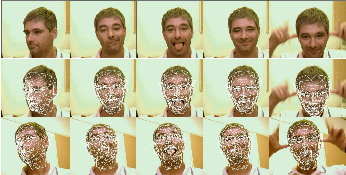
Figure 6: Stereo tracking result for Sequence B (320x240 @ 30 FPS); The first row shows the input images from the upper camera. The second and third rows show the projected face model overlaid on the images from the upper and lower camera, respectively. From left to right, the frame numbers are 56, 524, 568, 624, and 716.
