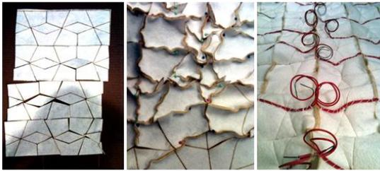
Figure 6. Laser cut felt, pinned felt, felt with sewn insulated Nitinol.
